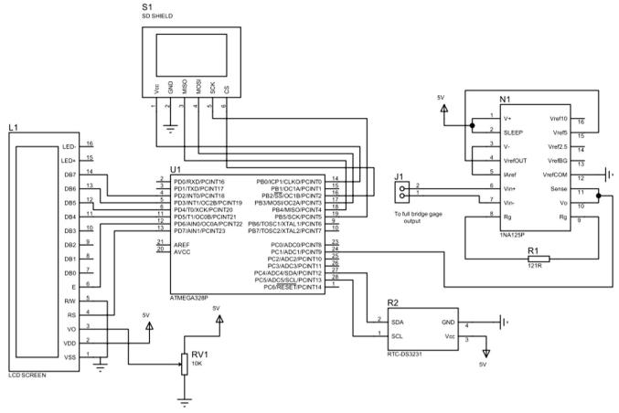
Fig. 1. TDV system control circuit schematic.
