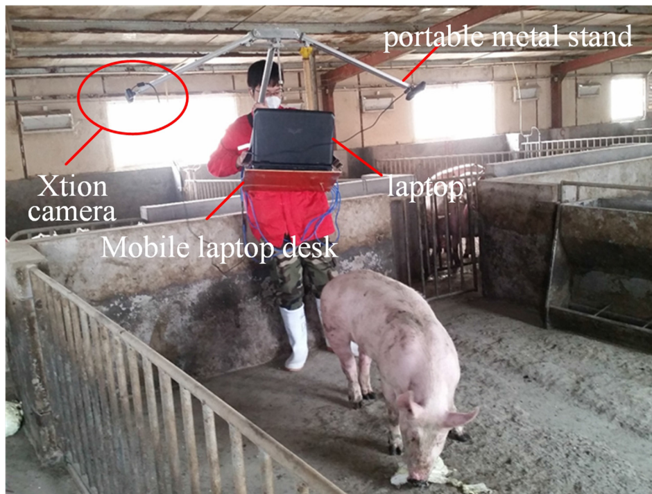
Fig. 1. Photo of the pig and the portable measurement system operated by the tester in the pig farm. The photo was taken in the daytime.
