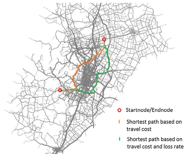
Fig. 3. Austin, Texas network. (With simulation of transport path based on costs) In Fig. 3, a graphical representation of the freely accessible network of Austin, Texas is presented. The figure indicates two possible simulations of apple transport in which the shortest path is calculated based on the travel cost (a) and based on both the travel cost and the loss rate of apples (b). Source Fig. 3: Barge, 2013.
