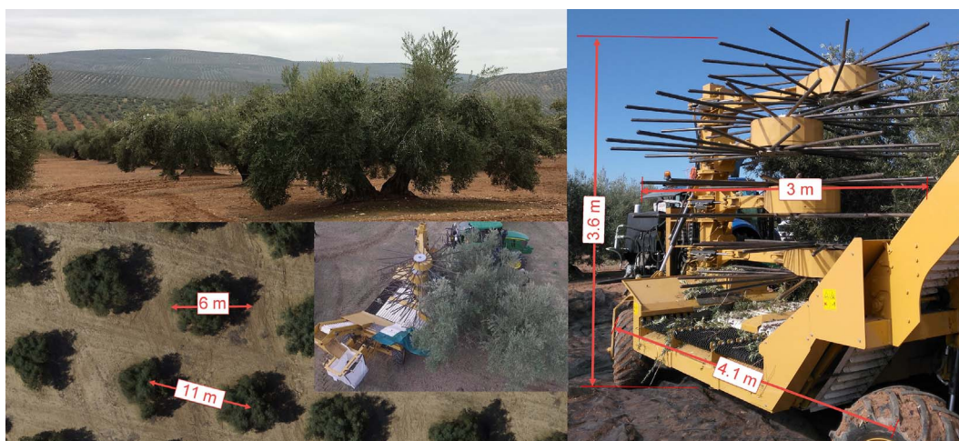
Fig. 1. Harvester with four canopy shaker heads for adapting to canopy olive trees.
