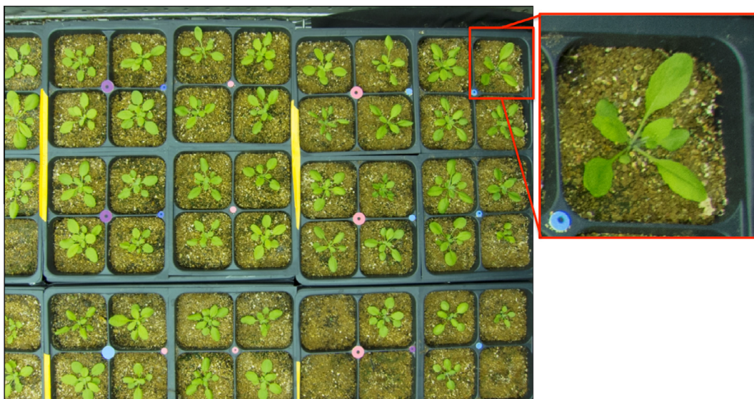
Fig. 1. Original image with optical distortion and perspective distortion. An original image from indoor environment showing plants before optical distortion and perspective distortion correction. The plants from the corners were seriously distorted and true distances and areas cannot be measured directly from the image.
