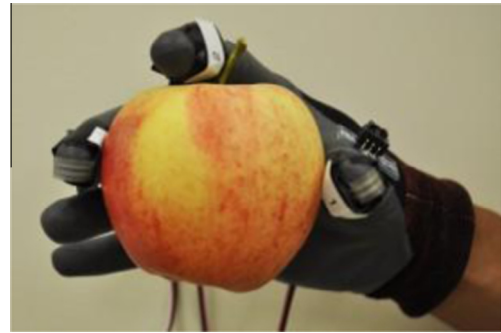
Fig. 1. Instrumentation glove used for evaluating picking motions (Sensor Model: GripTM, Tekscan, USA).
