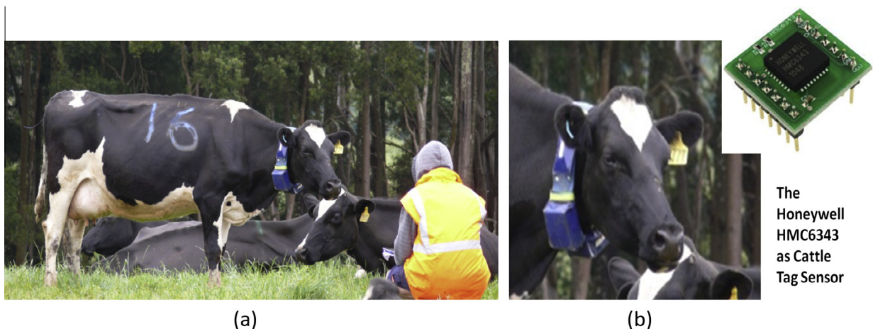
Fig. 1. (a) Cow 16 at the TIA Dairy Research Facility in Elliott, Tasmania, Australia. The sensor collar is attached around the cow's neck; (b) cattle collar sensor system for capturing motion patterns associated with behaviour.
