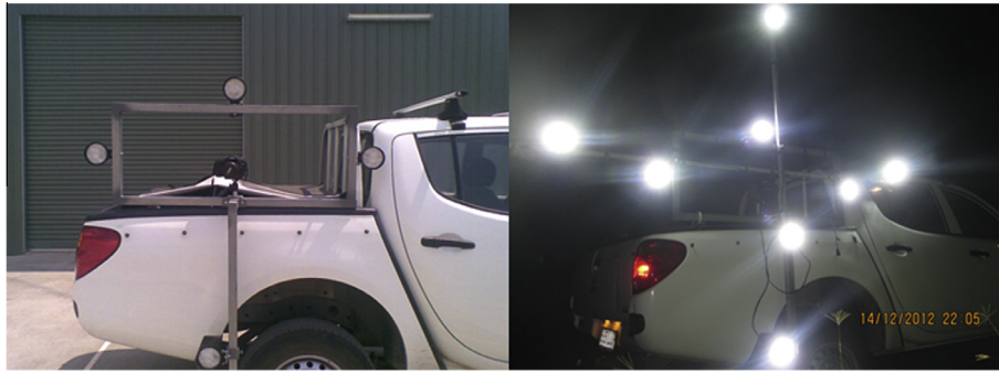
Fig. 1. Lighting rig as used for image collection. Left image shows rig as used in 2011 (day image). Right image shows rig as used in 2012 (fully illuminated). Only the inner four lights were illuminated during imaging for sets discussed in this paper to maintain consistency between sets.
