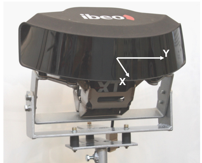
Fig. 2. Laser scanner ibeo ALASCA XT.
