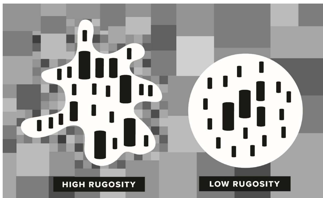
Fig. 1. Rugosity Visualization. Higher rugosity (left) and minimum rugosity (right) for the same urban area (shown in white with areas of greater density depicted as larger cylinders) as compared to the non-urban area (shown in grayscale). Higher urban rugosity can be achieved by maximizing the urban interface through implementation of greenbelts, green wedges, and wildlife habitat corridors. Higher densities on the urban interface are associated with smaller agricultural plot sizes and greater diversity of production. Image created by Nicole Martin of the Center for Regional Change.
