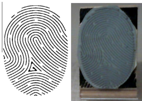
Fig. 1. Left: Artificial fingerprint artwork. This pattern was used to create a rubber stamp as described as in the text. Right: The custom rubber stamp used to create the transfer prints.
