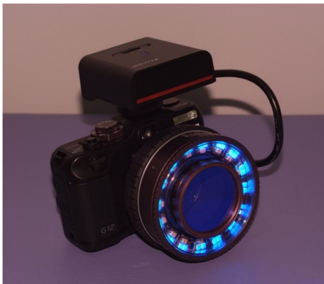
Fig. 1. Illuma-Light (a series of bright white and 470-nm blue LED lights that provide 360-degree shadow-free lighting; blue ring).
