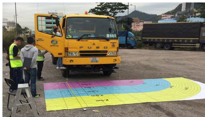
Fig. 1. The coloured plastic mat with grids used for measurement of field of view of the front blind spot mirror.
