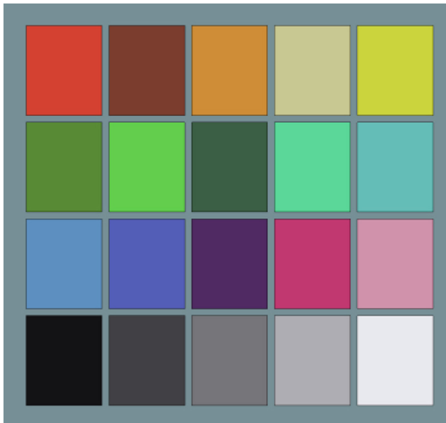
Fig. 1. The calibration chart by DSC Labs [13]. This chart has optimally placed colors for calibration.
