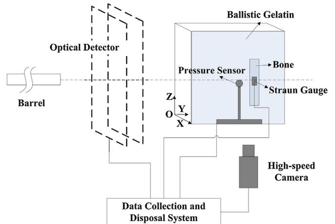
Fig. 4. Experiment set up.
