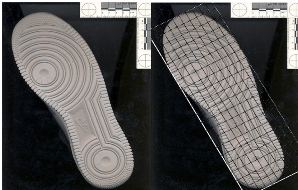
Fig. 1. (Left): Sole of the shoe used in the study showing artificial cut-marks cut into the sole using a dental drill, prior to any use of the shoe. (Right): The same image with the 200 cell grid superimposed on it.
