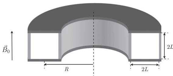
Fig. 1. Sketch of the annular geometry. The color of the walls indicates their electric conductivity: perfectly conducting (light gray), and perfectly insulating (dark gray).
