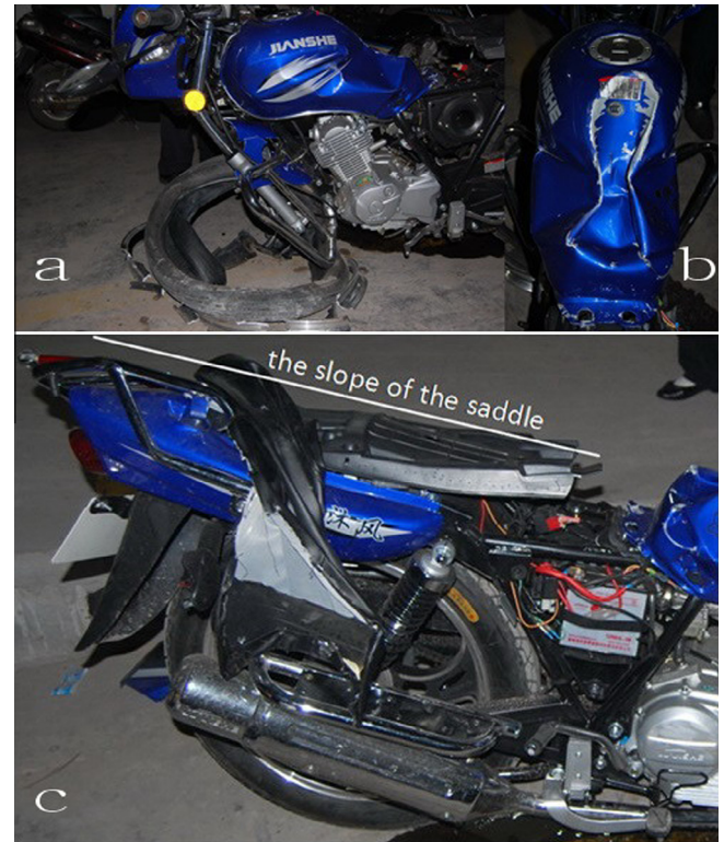
Fig. 2. The deformation of the motorcycle after impact (a) front wheel and front fork of the motorcycle (b) the fuel tank of the motorcycle (c) the slope on the surface of the saddle.
