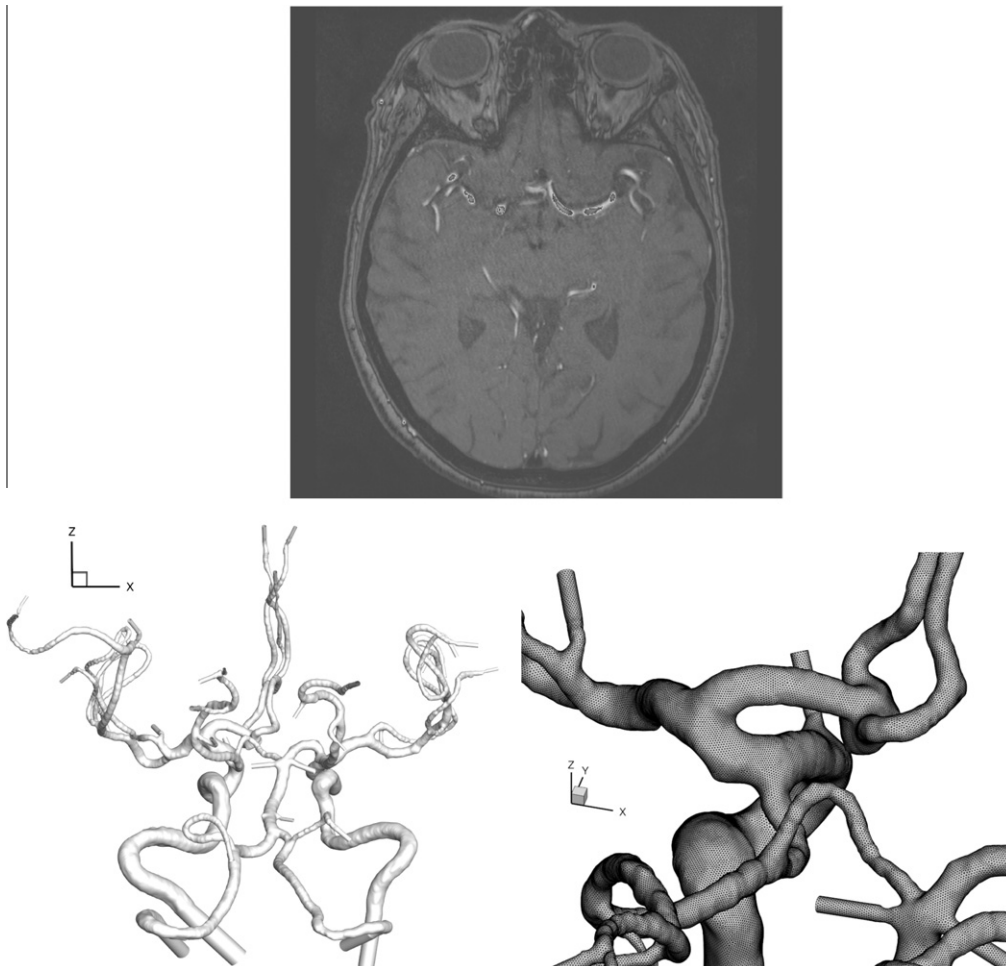
Fig. 1. Top-example of a raw MRI image with an enhanced contrast agent in the brain vascular system. White contrast indicates brain blood vessels in the particular horizontal slice. Bottom/left-reconstructed 3D geometry; Bottom/right-generated tetrahedral numerical mesh (a zoom-in).
