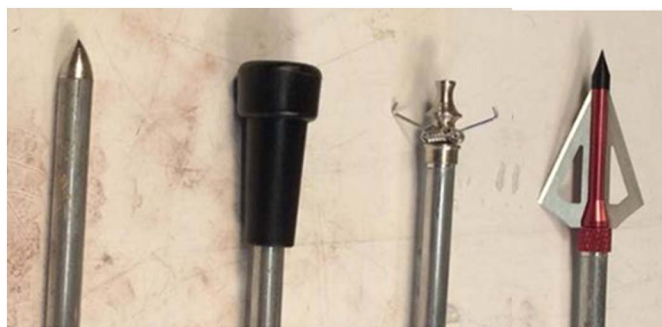
Fig. 1. Left to right: bullet, blunt, judo and broadhead arrowheads used during the project.
