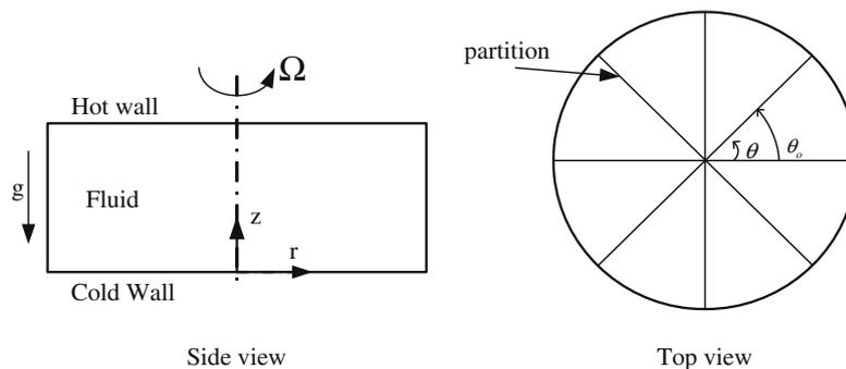
Fig. 1. Schematic of rotating cylinder with partitions.
