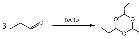
Scheme 1. Cyclotrimerization of propanal catalyzed by BAILs.
