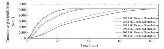
Fig. 2. Cumulative gas production over time for different stimulation temperatures. The thermal stimulation and combined methods were compared for different temperatures.
