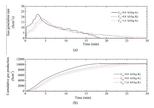
Fig. 3. (a) Gas generation rate and (b) cumulative gas production over time for different core specific heat capacities (C<sub>ps</sub>): 0, 0.8, and 1.6 kJ/(kg K).
