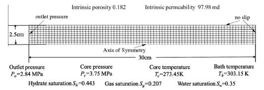
Fig. 1. Scheme of the computational hydrate core sample adapted from previous work [17-21].
