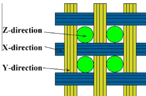
Fig. 1. Schematic of the fine-woven 3D composite preforms.
