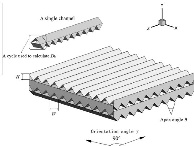
Fig. 1. Schematic of the section in the cross-corrugated exchanger.
