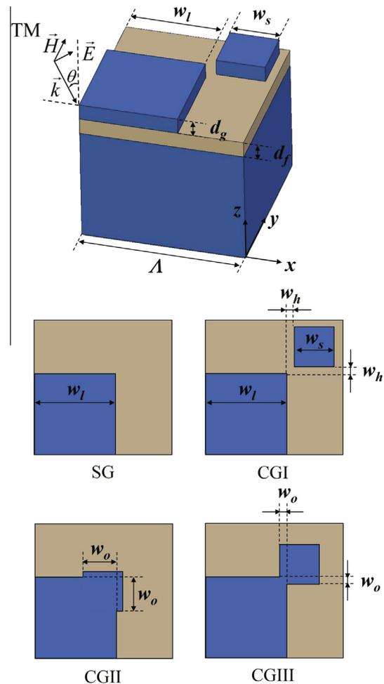
Fig. 1. Schematic of one unit cell of CGI and top view of four types of grating structures.
