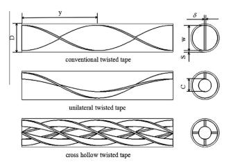
Fig. 1. Tube fitted with conventional, unilateral, and cross hollow twisted tapes.
