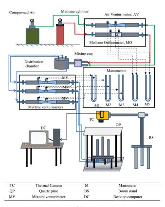
Fig. 1. Schematic of the experimental setup.
