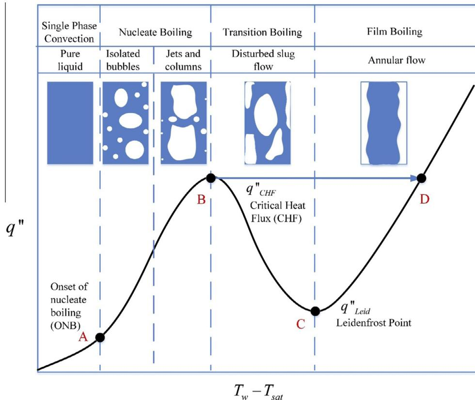
Fig. 1. A typical boiling curve including different boiling regimes and corresponding flow patterns.
