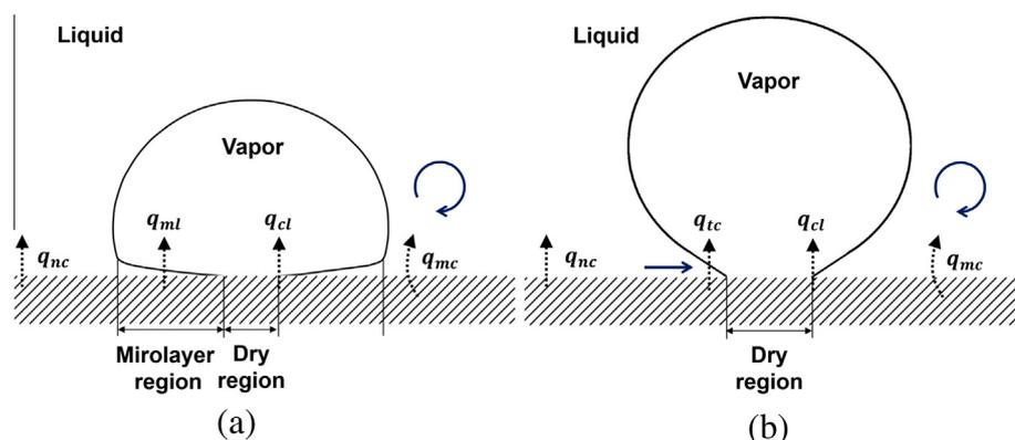
Fig. 1. Physical mechanisms of heat transfer during single-bubble nucleate boiling. (a) Bubble growth period and (b) bubble departure period.
