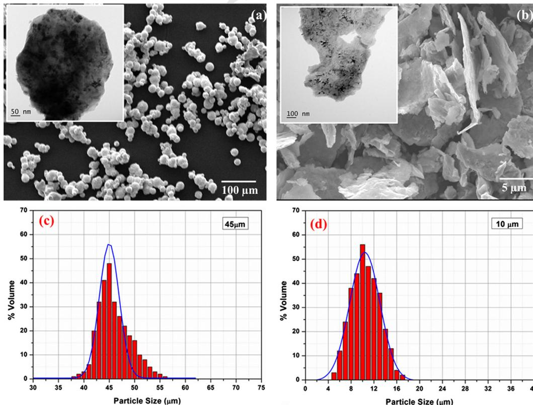
Fig. 2. SEM and PSA of NiTi powder elements with (a, c) 45 μm (b, d) 10 μm in size.
