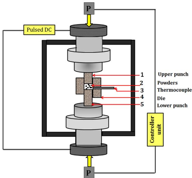
Fig. 1. Schematic view of SPS-setup.
