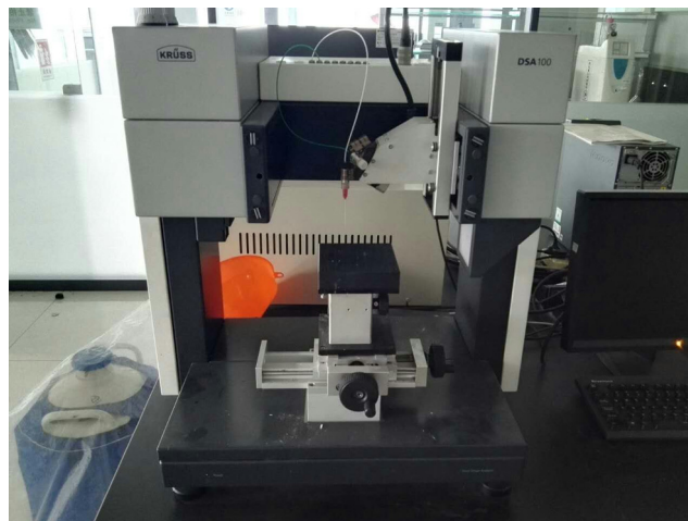
Fig. 2. KRÜSS DSA100 optical contact angle measuring instrument.
