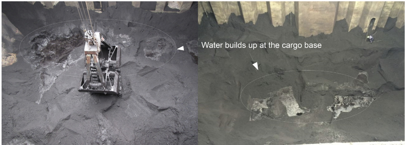
Fig. 1. Migrated water builds up at the base of the cargo hold after a shipping journey.
