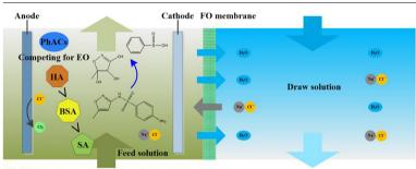
FO-EO: Simultaneous Rejection and Degradation of PhACs
