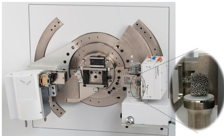
**Fig. 1.** Photography of the PANalytical Empyrean X-ray diffractometer operated in tomography mode: Molybdenum X-ray tube (left), rotatable sample stage with catalyst foam (zoomed inset) and GaliPIX<sup>3D</sup> detector (right).
