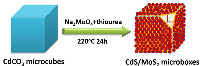
Fig. 1. Schematic illustration of the in-situ formation process of the CdS/ \text{MoS}_2 microboxes.
