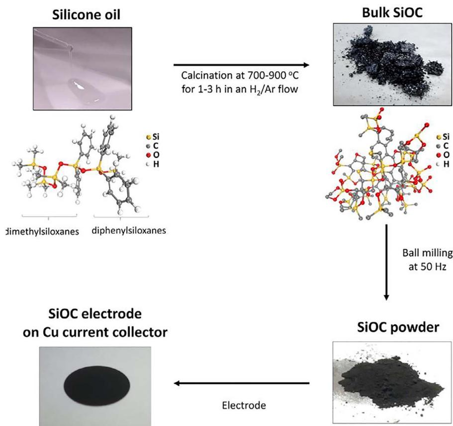
**Scheme 1.** A schematic of the synthesis procedure of SiOCs from silicone oil.
