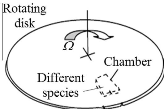
Fig. 1. Concept of rotating disk for microfluidic application.
