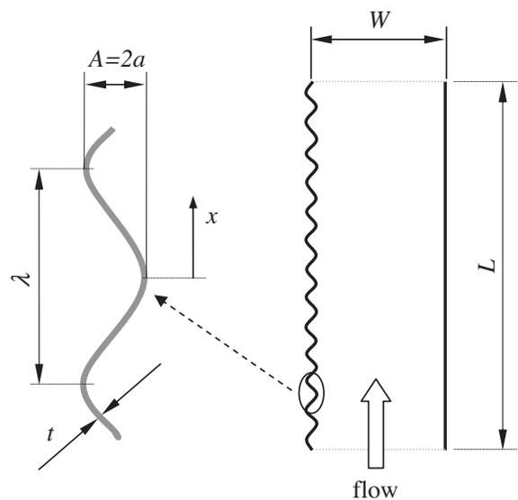
Fig. 1. Two-dimensional vertical channel with a wavy surface on the left-hand side and a flat wall on the right-hand side.
