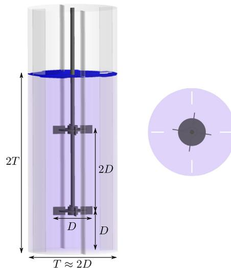
Fig. 1. Front and top views of the computational domain.
