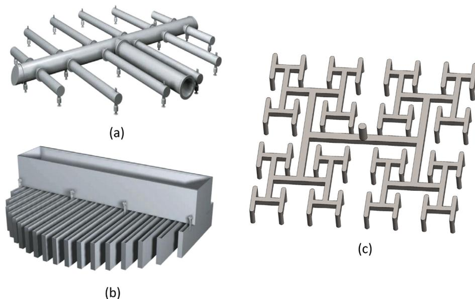
Fig. 1. (a) a conventional spray nozzle distributor (Sulzer Chemtech Ltd). (b) A trough-type liquid distributor (Sulzer Chemtech Ltd). (c) A fractal distributor.
