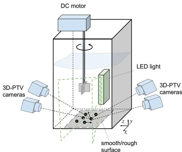
Fig. 1. Schematic view of the experimental set up: water tank, four-blade rotor, overhead stirrer driven by a DC motor, replaceable smooth or rough surfaces with the freely moving particles, four high speed digital cameras and LED line light source. The coordinate system is defined with the vertical y-axis.
