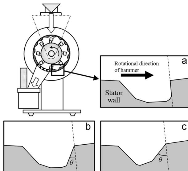
Fig. 2. Schematic of stator concaves with (a)  $\theta = 0$  deg, (b)  $\theta = 22.5$  deg, and (c)  $\theta = 45$  deg.
