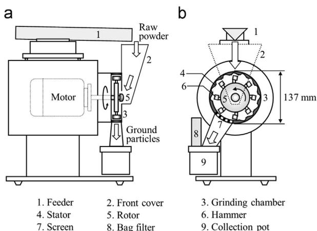
Fig. 1. Schematic of impact pulverizer. (a) side view (b) front view. 1. Feeder, 2. Front cover, 3. Grinding chamber, 4. Stator, 5. Rotor, 6. Hammer, 7. Screen, 8. Bag filter, 9. Collection pot.
