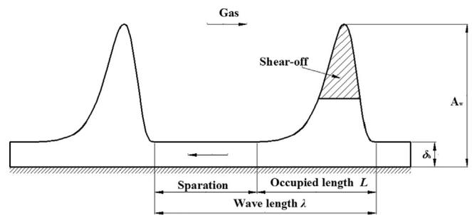
Fig. 2. Configuration of huge wave in churn flow.
