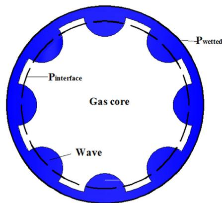
Fig. 3. Configuration of waves in churn flow.
