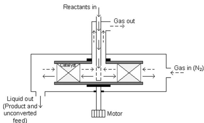
Fig. 1. Schematic of a solid catalyzed reactive HiGee stripper (SCRHS).
