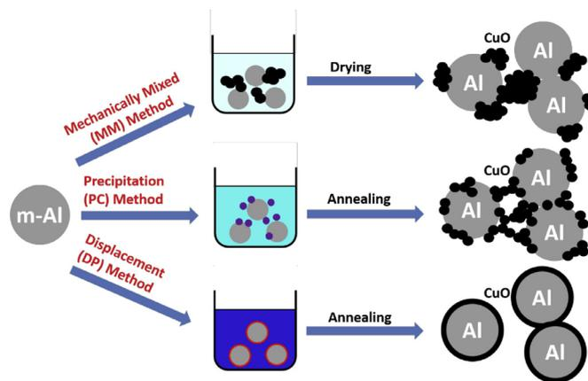
Fig. 1. The schematics of three different synthesis methods to prepare m-Al/CuO thermites and their expected morphologies.
