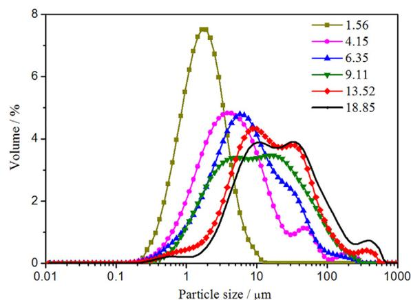
Fig. 1. Particle size distributions of NQ.
