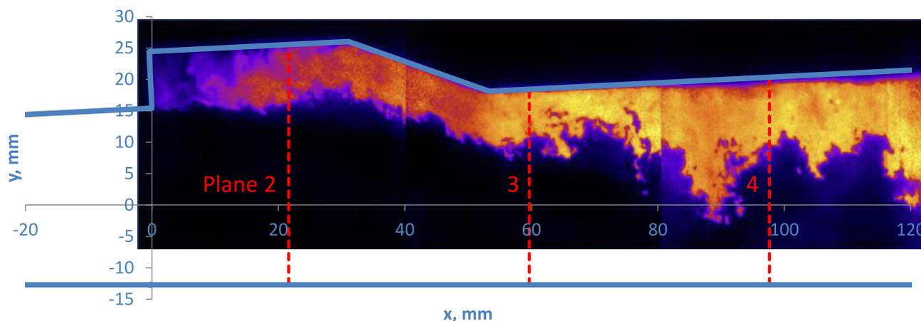
Fig. 1. Visualization of OH PLIF in the combustor, adapted from [1].
