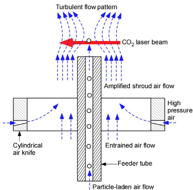
Fig. 2. Schematic diagram of the gas flow configuration in the experiments.
