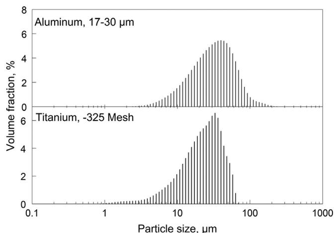
Fig. 1. Particle size distributions for aluminum and titanium powders used in experiments.
