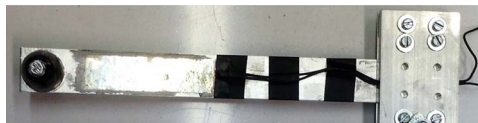
Fig. 1. An example of a piezoelectric cantilever type energy harvester deployed in the bridge.
